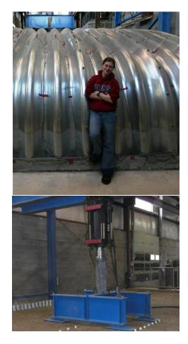
Surface load simulating tandem axle loads using the lab's 2000 kN actuator
